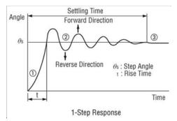
Vibration at low speeds is caused by a step-like movement that produces this type of damping oscillation. The vibration characteristics graph below represents the magnitude of vibration of a motor in rotation. The lower the vibration level, the smoother the motor rotation will be.
