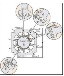
In other words, when excitation switches from phase A to B, the rotor rotates by 0.72°. As excitation shifts from phase A, to phases B, C, D and E, then back around to phase A, the stepping motor rotates precisely in 0.72° steps. To rotate in reverse, reverse the excitation sequence to phase A, E, D, C, B, then back around to phase A.
