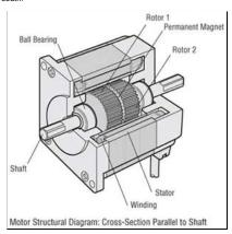
The stator has ten magnetic poles with small teeth, each pole being provided with a winding. Each winding is connected to the winding of the opposite pole so that both poles are magnetized in the same polarity when current is sent through the pair of windings. (Running a current through a given winding magnetizes the opposing pair of poles in the same polarity, i.e., north or south.)
