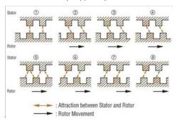
Stable Points: Points where the rotor stops, with the stator teeth and rotor teeth are exactly aligned. These points are extremely stable, and the rotor will always stop there if no external force is applied.
