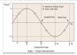
The following illustrations show the positional relationship between the rotor teeth and stator teeth at the numbered points in the diagram above. When held stable at point (1) the external application of a force to the motor shaft will produce torque T (+) in the left direction, trying to return the shaft to stable point (1). The shaft will stop when the external force equals this torque at point (2).
