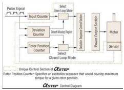
In the closed loop mode, motor-winding excitation is controlled so that maximum torque is developed for the given angular position of the rotor. This control method eliminates unstable points (misstep region) in the angle – torque characteristics.
